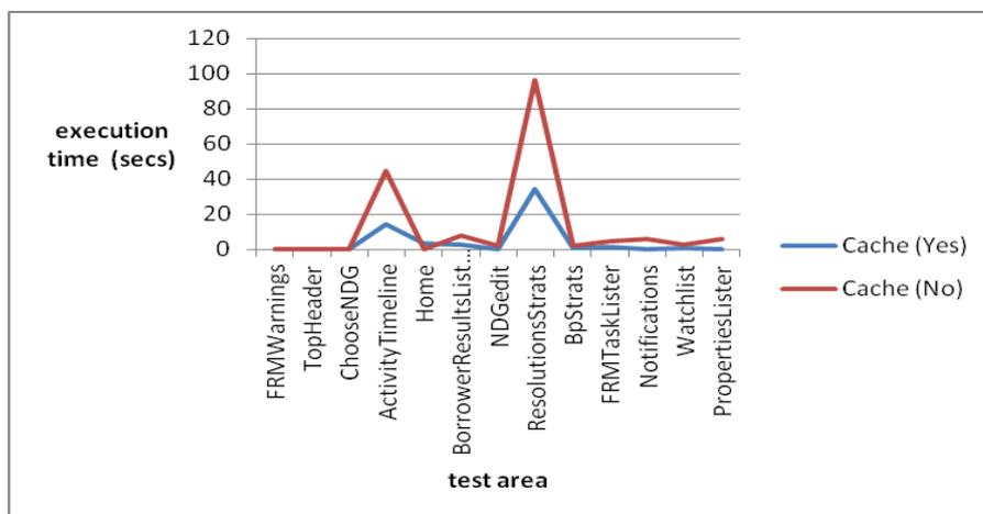
Fig.2 Graphic test results for 200000 records
