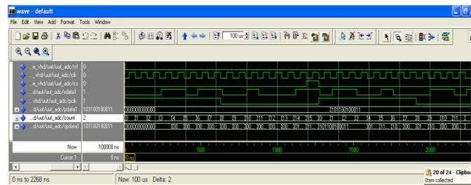
Figure-4: Simulation analog to digital converters (A/D) Interface
