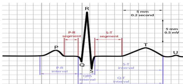
Fig.1 ECG signal characteristics
