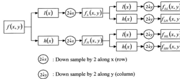
Figure 2. Discrete Wavelet Transform Archetcture
