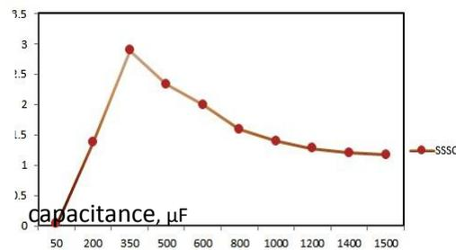
The above graph [39] shows reactive power improvement after compensating the system using SSSC. It is seen that reactive power improves only up to a certain value of capacitance (350 $\mu\text{F}$ ) beyond which it deteriorates.
