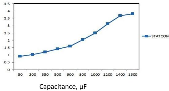
Figure 37: Variation of power flow with change in capacitance (50-1500 $\mu\text{F}$ )
