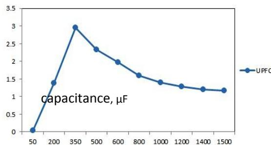
Figure 40: Variation of power flow with change in capacitance (50-1500 $\mu\text{F}$ )
