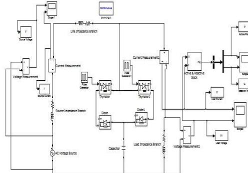
**Figure 16: STATCOM compensated system**
