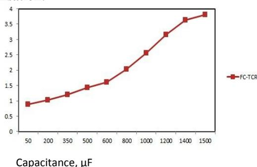
**Figure 36:** Variation of power flow with change in capacitance (50-1500 $\mu$ F)
