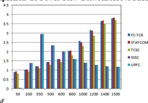
**Figure 41:** Variation of power flow between above FACTS devices with change in capacitance (50-1500 $\mu$ F)
