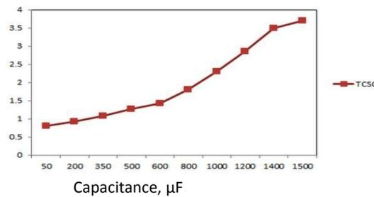
Figure 38: Variation of power flow with change in capacitance (50-1500 $\mu\text{F}$ )
