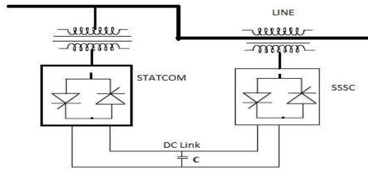
Figure 5: Unified power flow controller
