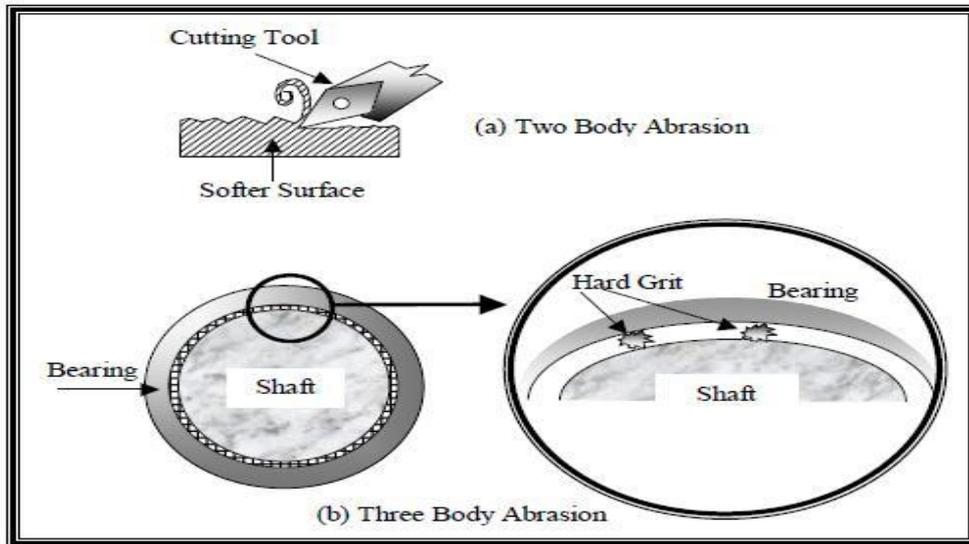
**Fig 2** Abrasive Wear
