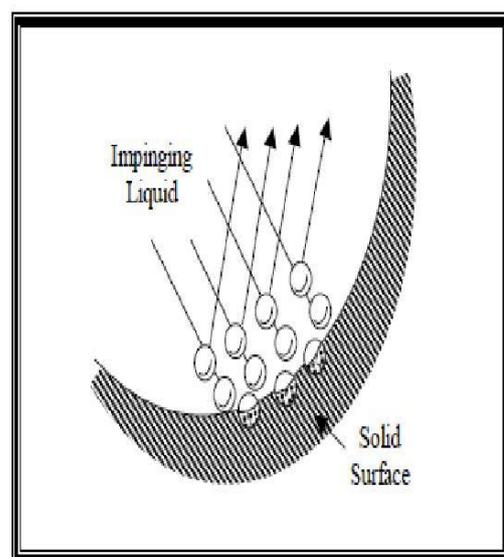
Schematic of cavitation erosion due to impingement of liquid bubbles.
