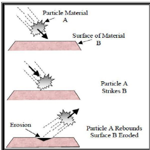
Schematic of erosive wear.
