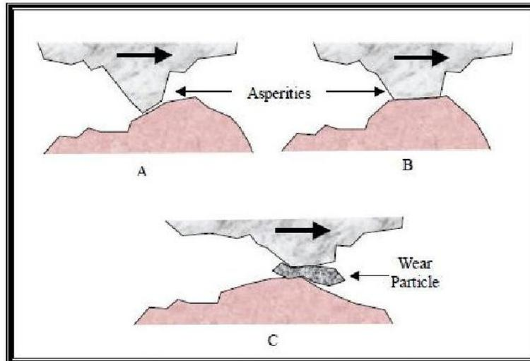
Schematic of generation of a wear particle as a result of adhesive wear process.
