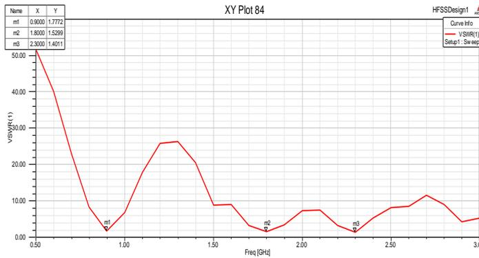
Fig. 14 simulated vswr for the dielectric height h=7.6
