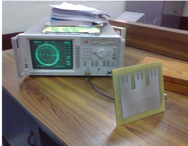
Fig 21 Antenna design with network analyser
