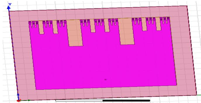
Fig.3, the pictorial representation of the proposed design for third iteration of E-shape fractal (3EFPA) is produced with optimized dimensions.
