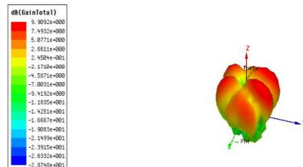
Fig. 20 simulated gain with the value of gain = 9.9db
