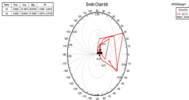
Fig. 15 simulated impedance chart
