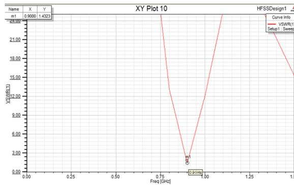
Fig. 6 simulated VSWR for first iteration.
