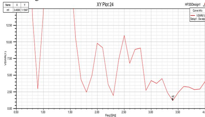
Fig. 18 simulated vswr for fourth iteration
