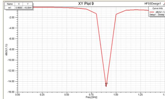
Fig. 5 simulated return loss for first iteration.
