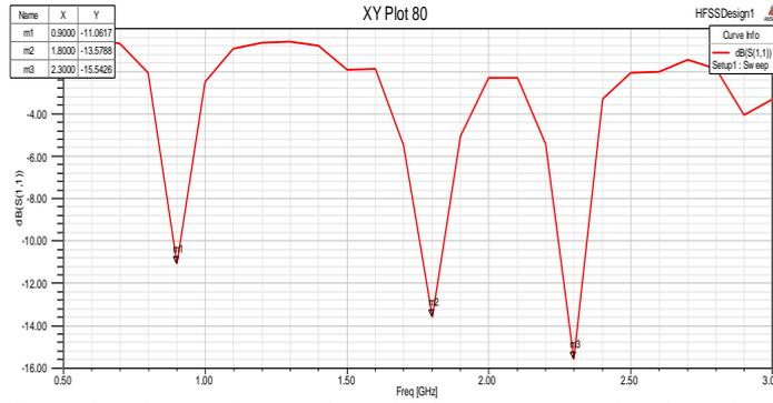
Fig. 13 simulated return loss with total h between ground and patch is h=7.6
