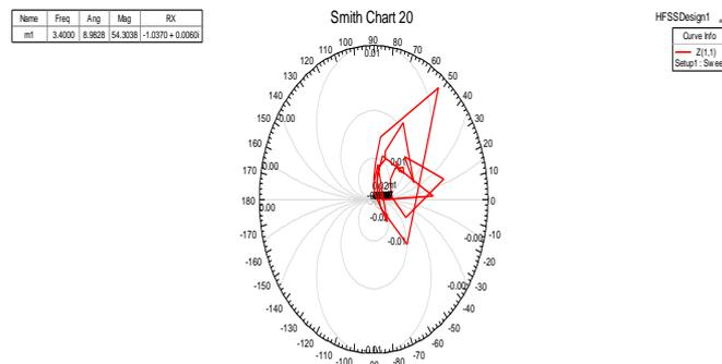
Fig. 19 simulated impedance chart for fourth iteration
