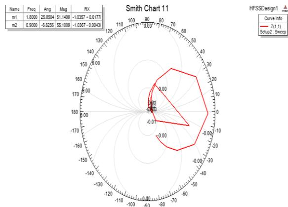
Fig. 11 simulated impedance for second iteration.
