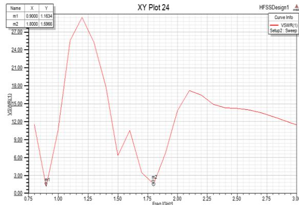
Fig. 10 simulated VSWR for second iteration.
