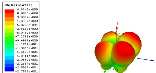
Fig. 16 simulated gain with the value of gain = 8.3db
