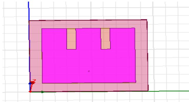
Fig.1, the pictorial representation of the proposed design for first iteration of E-shape fractal (1EFPA) is produced with optimized dimensions
