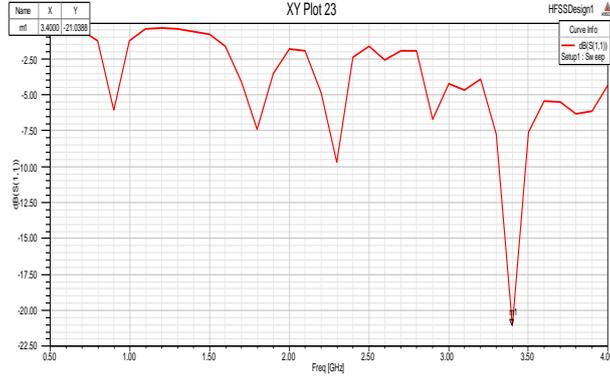
Fig.17 simulated return loss for fourth iteration
