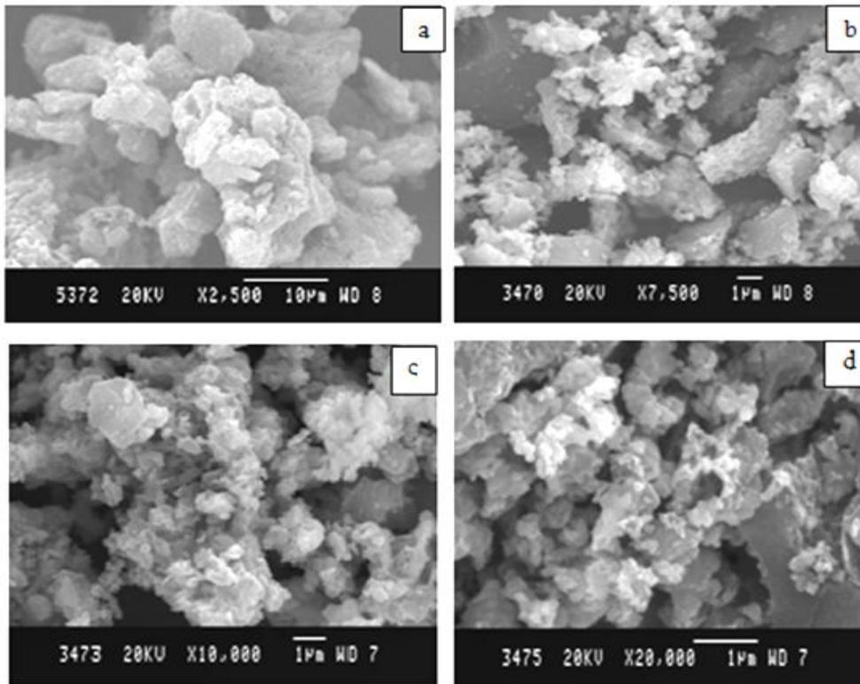
Figure 2 (a-d) show the SEM image of PANI and PANI/V<sub>2</sub>O<sub>5</sub> composites of different weight percentage (5, 15 and 25 wt %)
