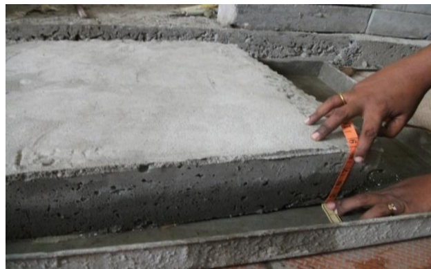
Figure 2 Measurements of water absorption in slab specimen
