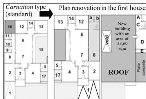
Figure 4: First house floor plan (survey 2012)
