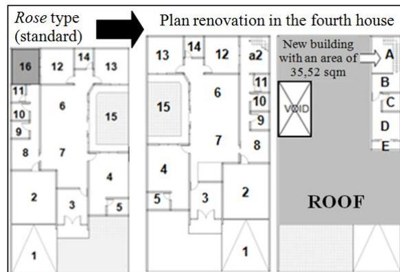
Figure 13: Fourth house floor plan (survey 2012)
