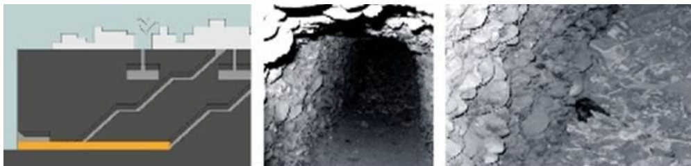
FIGURE 6: Shovadan Components: Horizontal Channels
