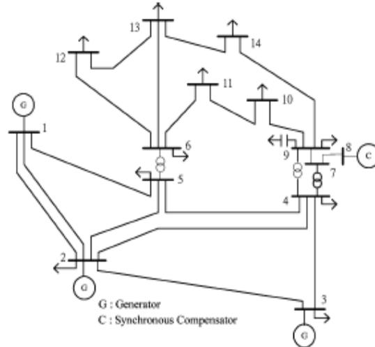
Fig.4 IEEE-14 test bus system
