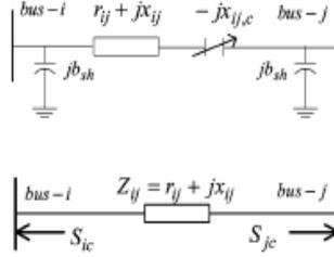
Fig. 2. Equivalent injection model of TCSC.
