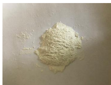
Figure 4: Sample of milled sodalime glass
