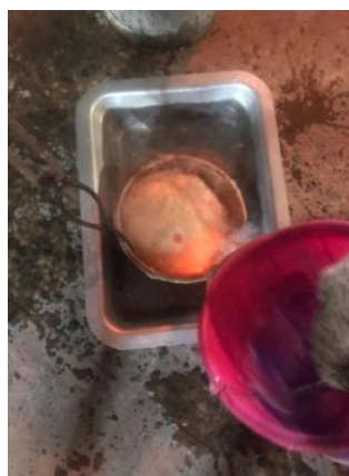
Figure 8: Composition poured in water for fritting
