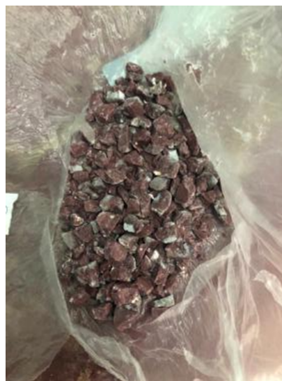
Figure 11: Samples of the glass frit composition after fritting
