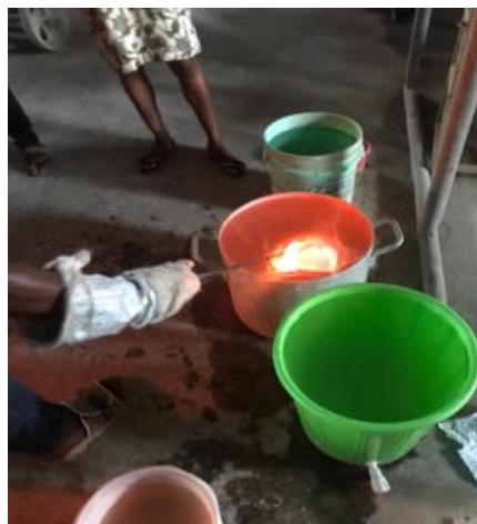
Figure 10: Composition poured in water to get the second frit.
