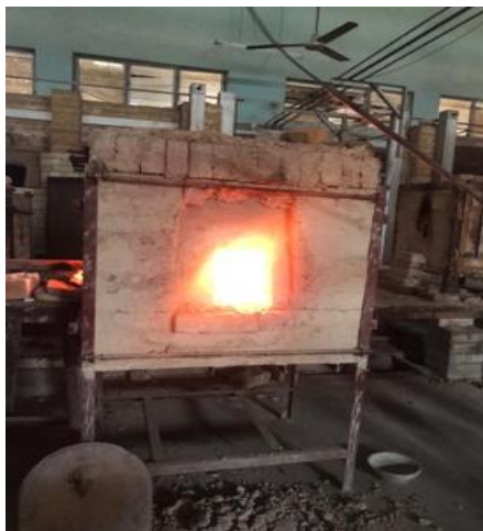
Figure 9: Sample in crucible placed in the Kiln for second firing.
