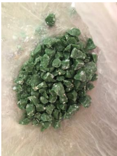
Figure 11: Samples of the glass frit composition after fritting
