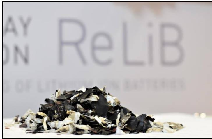
Figure 10. Batteries shredded in a separator used by Li-Cycle in Canada (Şocariciu, 2022).
