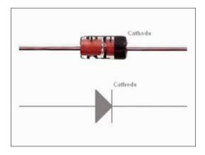
While seemingly simple, switching diodes like the 1N4148 DO-35 play a critical role in various electronic circuits, and our IoT-based smart notice board is no exception. This small but essential component offers specific functionalities that contribute to the overall system's operation. Here's a breakdown of why we incorporated the 1N4148 diode into our project:
