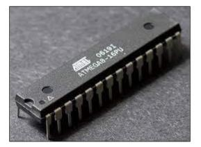
The core of our smart notice board system is the AVR ATmega8 microcontroller, specifically the DIP28 package variant. The ATmega8 is an 8-bit CMOS microcontroller from Microchip Technology, known for its low power consumption and versatile instruction set. Here's a breakdown of the key factors influencing our selection of the ATmega8 for this project:
