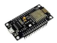
The ESP8266 is a key component enabling our smart notice board to connect to a Wi-Fi network and achieve remote communication. This highly-integrated chip from Espressif Systems offers a cost-effective and feature-rich solution for wireless connectivity in IoT projects. Here's a closer look at the factors that influenced our decision to utilize the ESP8266 in this project:
