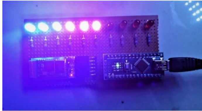
Figure 3. Displaying the attention level with an electronic circuit (LED circuit, each of which corresponds to 10% attention level)
