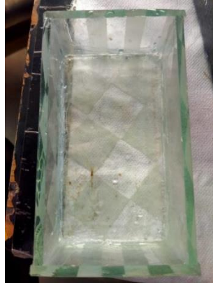
Fig-4. Glass Mould used for the preparation of specimen
