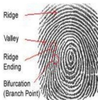
Figure. 1: Basic Types of Minutiae in Fingerprints
