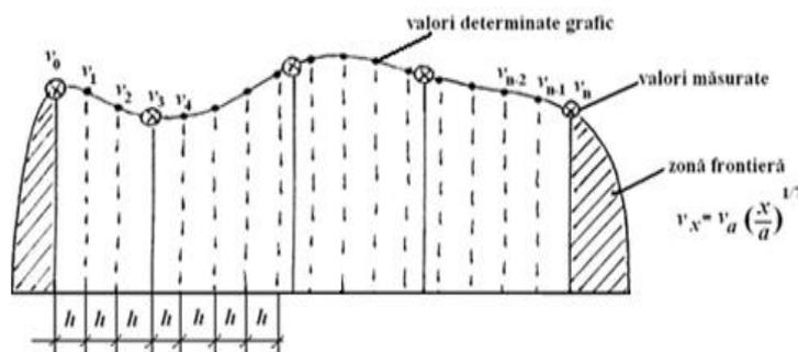
The determination of the average velocity and of the discharge, implicitly, by means of Simpson's rule can be carried out both graphically (Figure 3) and numerically, through the development of a computation program.
