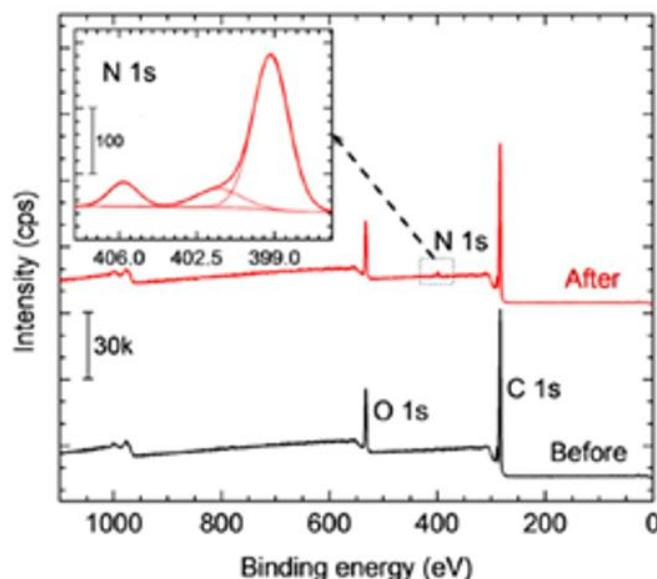
**Figure 2.** XPS survey spectra of pristine Plexiglas® before (black) and after (red) functionalization through nitrophenyl-vinylpyridine organic layer with the inset showing high resolution N 1s spectrum of the functionalized Plexiglas.
