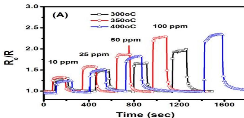
Fig 2: LPG sensing properties of the ZrO<sub>2</sub>
