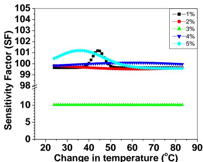
Fig 1. Variation of Sensitivity with change in operating temperature for different 1, 2, 3, 4, 5 wt% modified samples (1000 ppm LPG)
