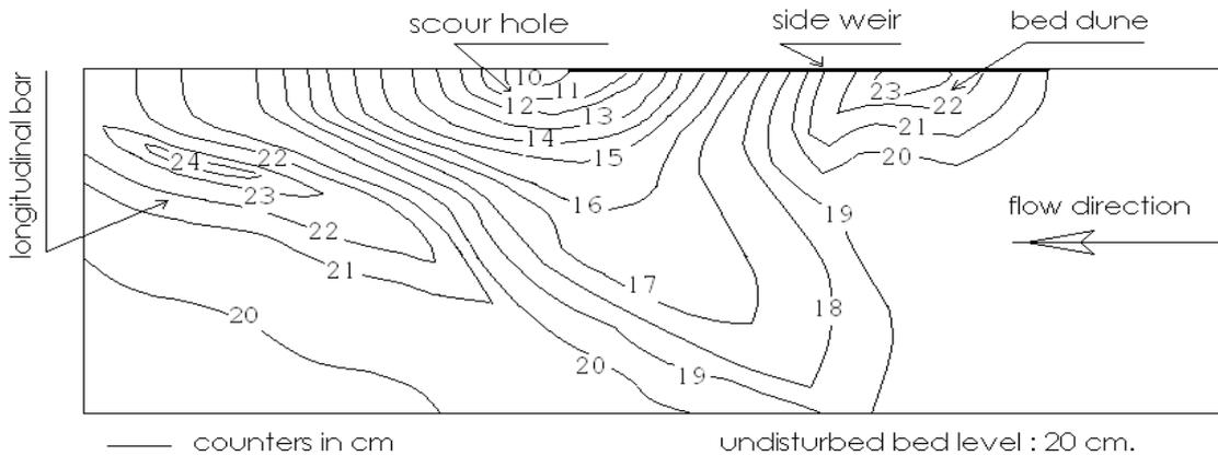
In this study, the scour depths around the side weir in moving-alluvial rivers were modeled mathematically using genetic programming. In addition, the accuracy of the mathematical models will be determined by comparing the scour depths measured in the physical model with the results of the GEP model.
