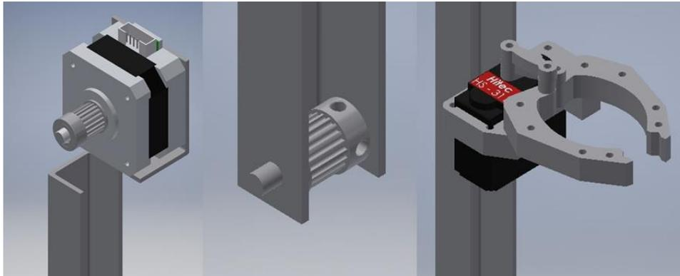
The complete mechanism that performs all the movement of the prototype is composed of two toothed pulleys with a distance between the center of 700 mm, a toothed belt that makes the connection between the two, a stepper motor that moves the assembly and a robotic claw ran through a motor.
