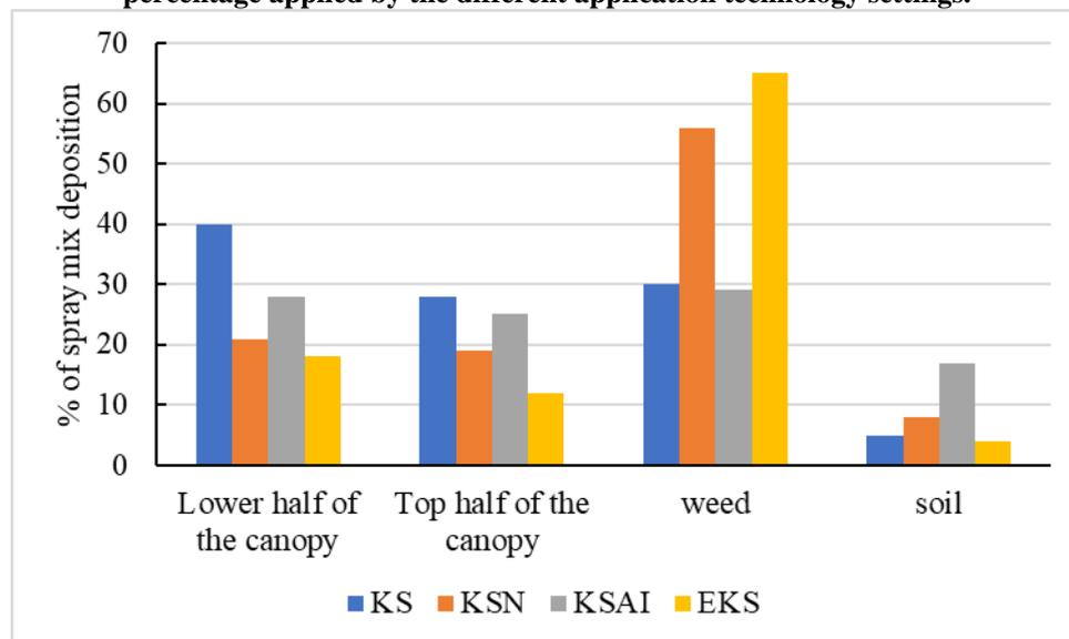
KSAI = knapsack sprayer with air induction nozzle; KS = knapsack sprayer; KSN = knapsack sprayer with Napoleon's hat; EKS = electrostatic sprayer.
