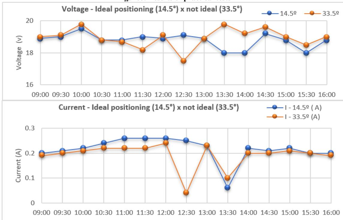
With the experimental data obtained, it is possible to calculate what the energy generated by this system will be and thus compares it with the theoretical values, and it is importante to highlight that the sudden peaks (see Figure 8) occurred due to the presence of clouds during the measurement, which drastically reduces the energetic potential of the photovoltaic panels due to shadowing. The local irradiance value was obtained by
