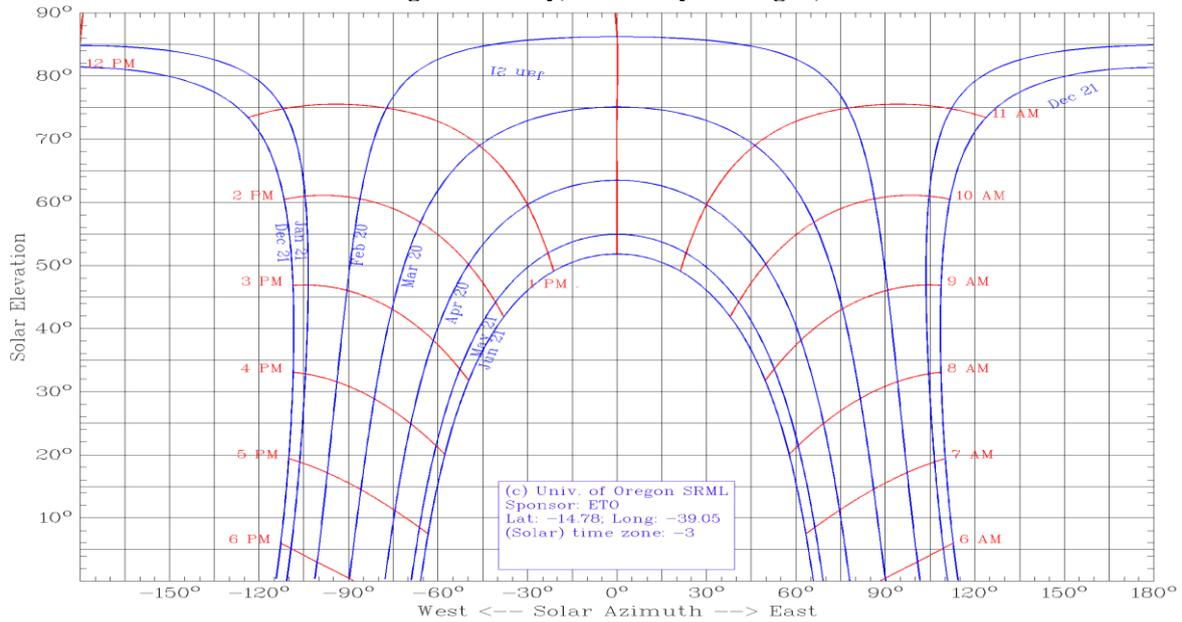
For the positioning of photovoltaic panels, the slope of the optimum surface,  $\beta_{opt}$ , is usually considered equal to the latitude of the place ( $\phi$ ) (CARNEIRO, 2009), and the amount of irradiance received in the panels can be calculated using Equation 2:
