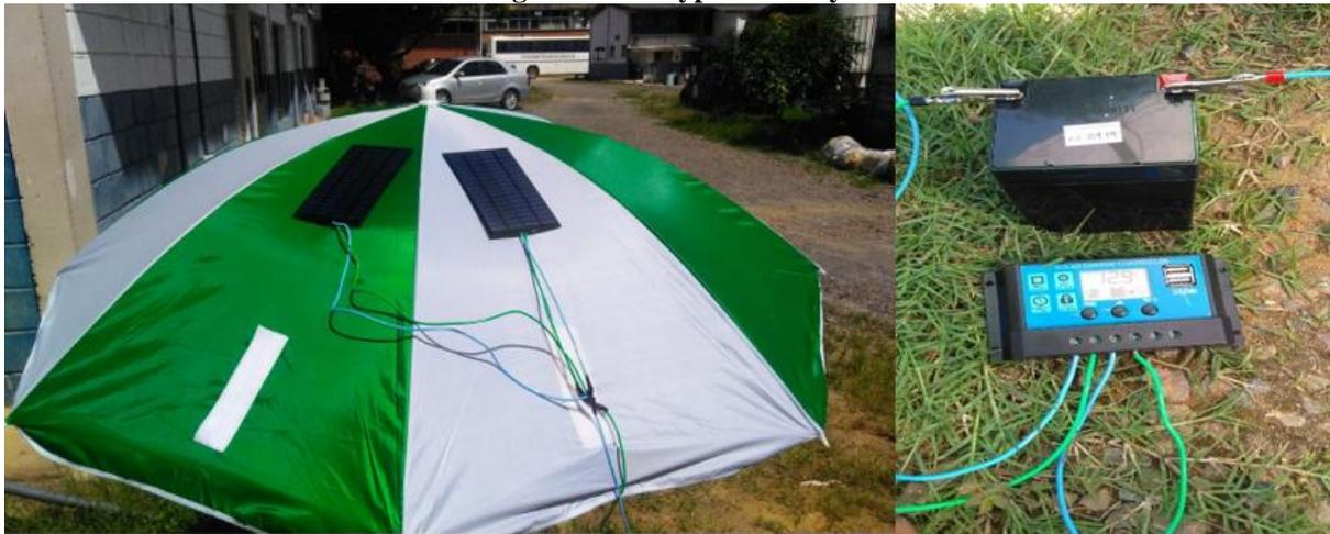
Using this test prototype, it was measured the temperature at the lower base of the panels at different intervals, with the aid of the thermometer Instrutherm TE-400. Another point analyzed is the positioning of the panels, as it interferes directly with the performance. Two positions were selected, one ideal, with an angle of approximately  $14.5^\circ$  (which can be seen on Figure 7) and the other not ideal, with approximately  $33.5^\circ$ .
